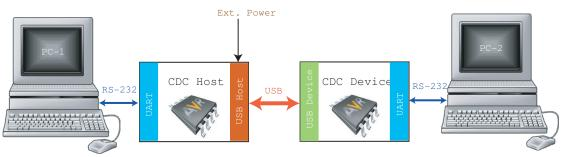
Note: Additional CDC device boards can be used to provide RS232 ports on the PCs if they only have USB ports available.
